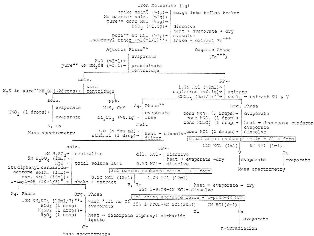
Fig. 3. Schematic diagram for the chemical separations of K, Ca, Ti, V, Cr and Mn from each other and from the target materials Fe, Ni and Co.
